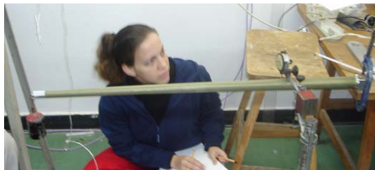
Figure 36: Tail Boom NDT Test.
